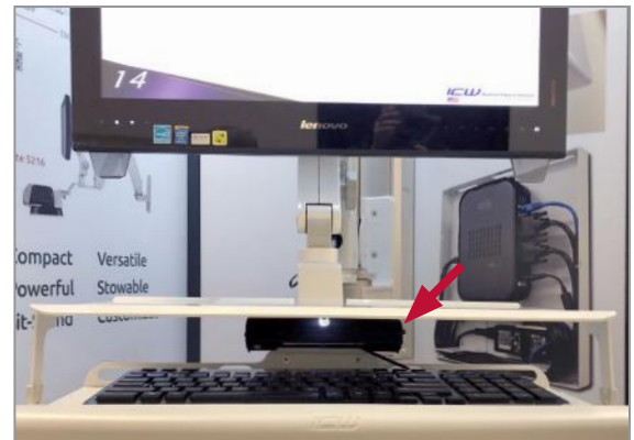
The UV-CLEAN self-disinfecting light is equipped with a sensor that activates once the surface has been contaminated in addition to its automated cleaning cycle system. When the user's hand comes near the light's sensor, the system deactivates.
